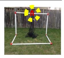
Slide uprights over stumps. Uprights are inserted into fat tubes already. Leave there. Top bar is exactly same as the bottom bar: 2 thin tubes into 1 fat tube. (1 is already inserted) MESH: Tie red strap in middle.
